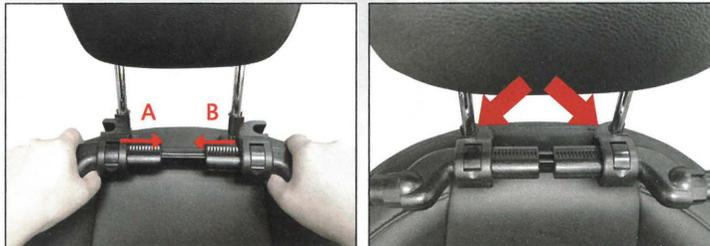
2. Insert the A end of the mounting rod into the B end, and hook the metal rod firmly on the headrest of the car
